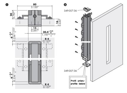
The lower end of the profile is marked with "profile below".
